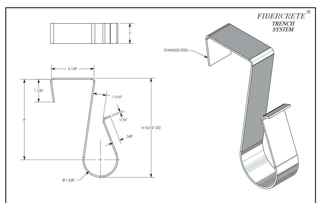
CHANNELS ARE NOTCHED FOR GROUND CABLE CLIPS.
