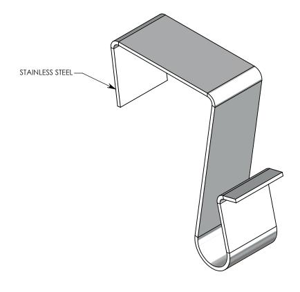
CHANNELS ARE NOTCHED FOR GROUND CABLE CLIPS.
