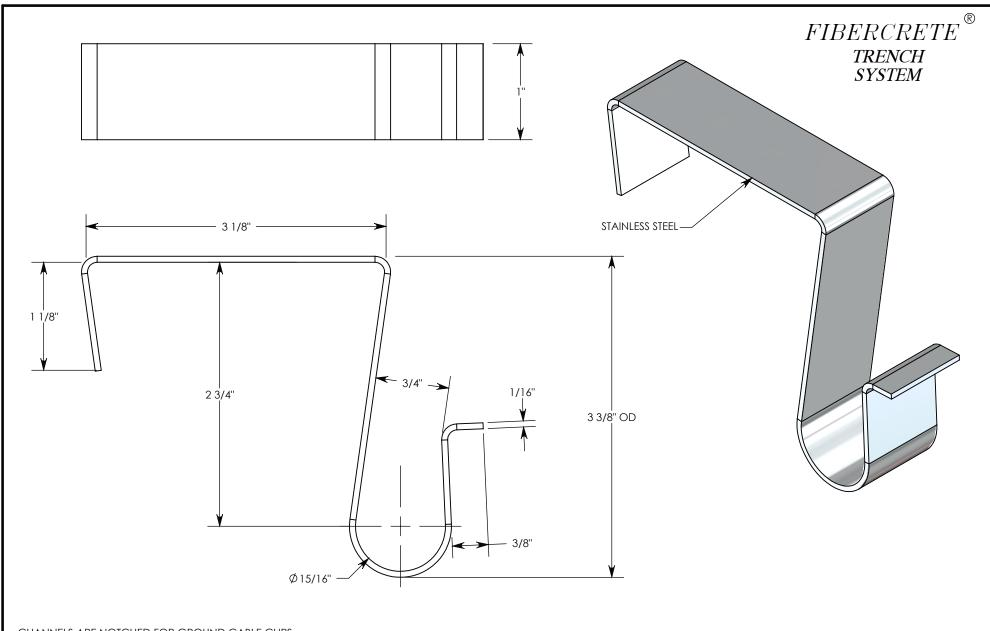
CHANNELS ARE NOTCHED FOR GROUND CABLE CLIPS.
