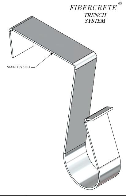
CHANNELS ARE NOTCHED FOR GROUND CABLE CLIPS.
