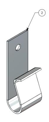
NOTE 1: .25" X 1.25" LONG CONCRETE SCREW INCLUDED (NOT SHOWN) NOTE 2: REQUIRES ONSITE DRILLING FOR INSTALLATION
