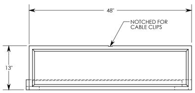
NOTE: FOR NON-STANDARD LENGTHS THE CHANNEL WILL BE SOLID BOTTOM AND DESIGNATED WITH ITS CORRESPONDING LENGTH MEASUREMENT. IE: 8010 32"
