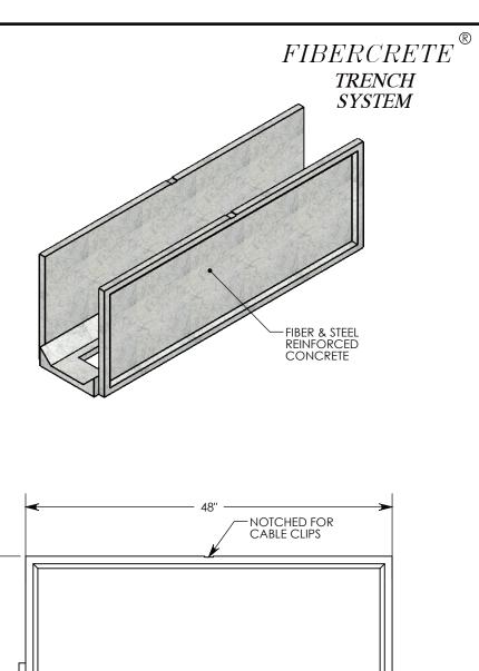
NOTE: FOR NON-STANDARD LENGTHS THE CHANNEL WILL BE SOLID BOTTOM AND DESIGNATED WITH ITS CORRESPONDING LENGTH MEASUREMENT. IE: 801016 32"
