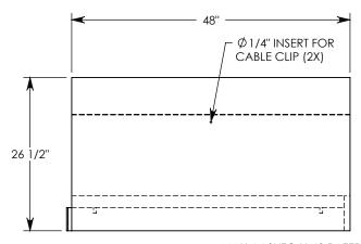
**NOTE 1:** FOR NON-STANDARD LENGTHS THE CHANNEL WILL BE DESIGNATED WITH ITS CORRESPONDING LENGTH MEASUREMENT. IE: 801016HT 32"
