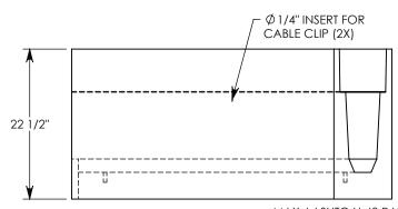
MAX AASHTO H-40 RATED - 64,000 LB. SINGLE AXLE LOAD DEPENDENT ON TRENCH COVER RATING MINIMUM ALLOWABLE SOIL BEARING PRESSURE – H-40: 5,500 PSF; H-20: 3,000 PSF
