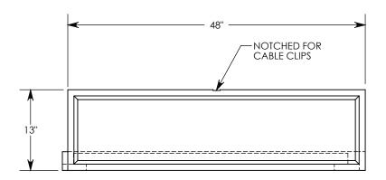
NOTE: FOR NON-STANDARD LENGTHS THE CHANNEL WILL BE SOLID BOTTOM AND DESIGNATED WITH ITS CORRESPONDING LENGTH MEASUREMENT. IE: 8020 32"
