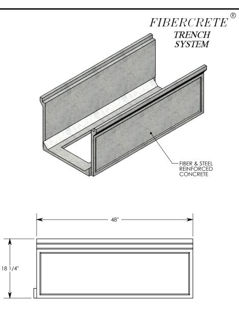
NOTE: FOR NON-STANDARD LENGTHS THE CHANNEL WILL BE SOLID BOTTOM AND DESIGNATED WITH ITS CORRESPONDING LENGTH MEASUREMENT. IE: 802016F 32"
