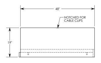
**NOTE:** FOR NON-STANDARD LENGTHS THE CHANNEL WILL BE SOLID BOTTOM AND DESIGNATED WITH ITS CORRESPONDING LENGTH MEASUREMENT. IE: 802016PTSB 32"
