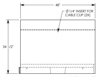
NOTE 1: FOR NON-STANDARD LENGTHS THE CHANNEL WILL BE SOLID BOTTOM AND DESIGNATED WITH ITS CORRESPONDING LENGTH MEASUREMENT. IE: 802024HT 32"
