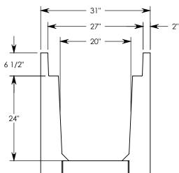
GALV. STEEL TOP RAILS STEEL REINFORCED CONCRETE
