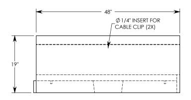
**NOTE 1:** FOR NON-STANDARD LENGTHS, THE CHANNEL WILL BE SOLID BOTTOM AND DESIGNATED WITH ITS CORRESPONDING LENGTH MEASUREMENT. IE: 8020HT3 32"
