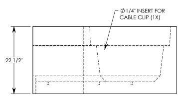
MAX AASHTO H-40 RATED - 64,000 LB. SINGLE AXLE LOAD DEPENDENT ON TRENCH COVER RATING MINIMUM ALLOWABLE SOIL BEARING PRESSURE – H-40: 4,000 PSF; H-20: 3,000 PSF
