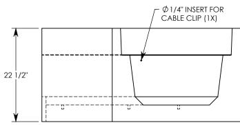
MAX AASHTO H-40 RATED - 64,000 LB. SINGLE AXLE LOAD DEPENDENT ON TRENCH COVER RATING MINIMUM ALLOWABLE SOIL BEARING PRESSURE – H-40: 4,000 PSF; H-20: 3,000 PSF
