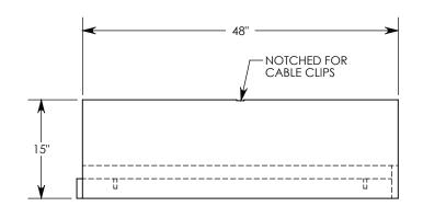
**NOTE:** FOR NON-STANDARD LENGTHS THE CHANNEL WILL BE SOLID BOTTOM AND DESIGNATED WITH ITS CORRESPONDING LENGTH MEASUREMENT. IE: 8020PTSB 32"
