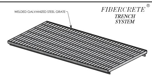
COVER ASSEMBLES ONTO 20" INSIDE WIDTH PEDESTRIAN RATED CONCAST CHANNEL.
