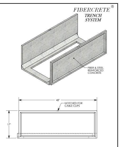
NOTE: FOR NON-STANDARD LENGTHS THE CHANNEL WILL BE SOLID BOTTOM AND DESIGNATED WITH ITS CORRESPONDING LENGTH MEASUREMENT. IE: 802416 32"
