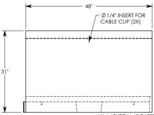
MAX AASHTO H-40 RATED - 64,000 LB. SINGLE AXLE LOAD DEPENDENT ON TRENCH COVER RATING MINIMUM ALLOWABLE SOIL BEARING PRESSURE – H-40: 3,500 PSF; H-20: 3,000 PSF
