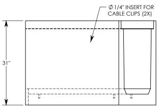
MAX AASHTO H-40 RATED - 64,000 LB. SINGLE AXLE LOAD DEPENDENT ON TRENCH COVER RATING
