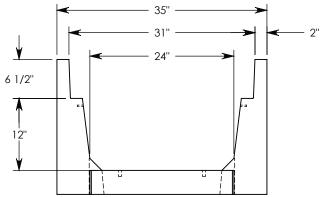
**NOTE 1:** FOR NON-STANDARD LENGTHS THE CHANNEL WILL BE SOLID BOTTOM AND DESIGNATED WITH ITS CORRESPONDING LENGTH MEASUREMENT. IE: 8024HT 32"
