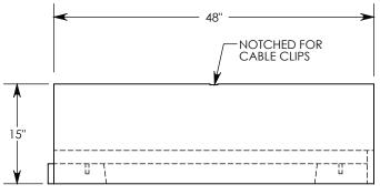
**NOTE:** FOR NON-STANDARD LENGTHS THE CHANNEL WILL BE SOLID BOTTOM AND DESIGNATED WITH ITS CORRESPONDING LENGTH MEASUREMENT. IE: 8024PT 32"
