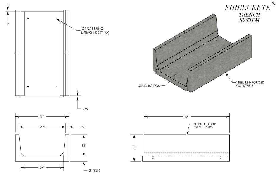
**NOTE:** FOR NON-STANDARD LENGTHS THE CHANNEL WILL BE SOLID BOTTOM AND DESIGNATED WITH ITS CORRESPONDING LENGTH MEASUREMENT. IE: 8024PTSB 32"
