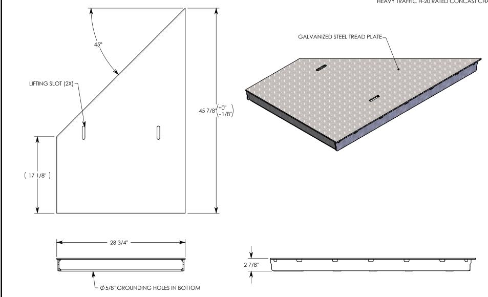
NOTE 1: FOR NON-STANDARD LENGTHS, THE PART NUMBER WILL CORRESPOND TO IT'S MEASURED LENGTH. IE: 8025HTSG 45L 18"
