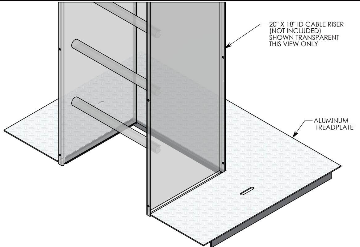
COVER ASSEMBLES ONTO 24" INSIDE WIDTH LIGHT TRAFFIC RATED CONCAST LT CHANNEL.
