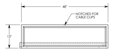
NOTE: FOR NON-STANDARD LENGTHS THE CHANNEL WILL BE SOLID BOTTOM AND DESIGNATED WITH ITS CORRESPONDING LENGTH MEASUREMENT. IE: 8030 32"
