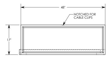
NOTE: FOR NON-STANDARD LENGTHS THE CHANNEL WILL BE SOLID BOTTOM AND DESIGNATED WITH ITS CORRESPONDING LENGTH MEASUREMENT. IE: 803016 32"
