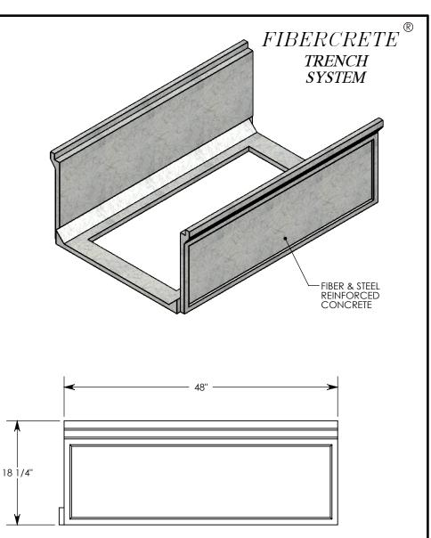
NOTE: FOR NON-STANDARD LENGTHS THE CHANNEL WILL BE SOLID BOTTOM AND DESIGNATED WITH ITS CORRESPONDING LENGTH MEASUREMENT. IE: 803016F 32"
