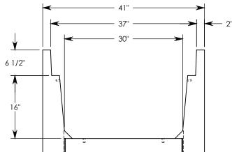
**NOTE 1:** FOR NON-STANDARD LENGTHS THE CHANNEL WILL BE SOLID BOTTOM AND DESIGNATED WITH ITS CORRESPONDING LENGTH MEASUREMENT. IE: 803016HT 32"
