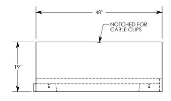
**NOTE:** FOR NON-STANDARD LENGTHS THE CHANNEL WILL BE SOLID BOTTOM AND DESIGNATED WITH ITS CORRESPONDING LENGTH MEASUREMENT. IE: 803016PT 32"
