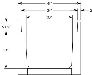
**NOTE 1:** FOR NON-STANDARD LENGTHS THE CHANNEL WILL BE SOLID BOTTOM AND DESIGNATED WITH ITS CORRESPONDING LENGTH MEASUREMENT. IE: 803024HT 32"
