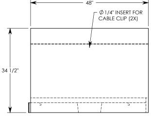
MAX AASHTO H-40 RATED - 64,000 LB. SINGLE AXLE LOAD DEPENDENT ON TRENCH COVER RATING MINIMUM ALLOWABLE SOIL BEARING PRESSURE – H-40: 3,000 PSF; H-20: 3,000 PSF
