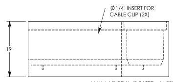
MAX AASHTO H-40 RATED - 64,000 LB. SINGLE AXLE LOAD DEPENDENT ON TRENCH COVER RATING MINIMUM ALLOWABLE SOIL BEARING PRESSURE – H-40: 3,000 PSF; H-20: 3,000 PSF
