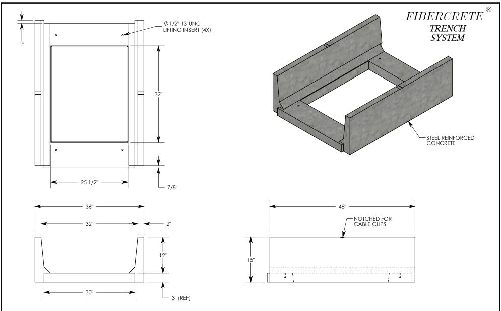
**NOTE:** FOR NON-STANDARD LENGTHS THE CHANNEL WILL BE SOLID BOTTOM AND DESIGNATED WITH ITS CORRESPONDING LENGTH MEASUREMENT. IE: 8030PT 32"
