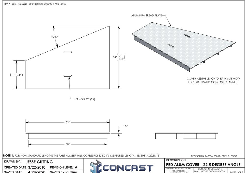
4/28/2020 SAVED DATE: SAVED BY: jgutting WEIGHT: MATERIAL: 19 LBS. **WELDED ALUMINUM**
