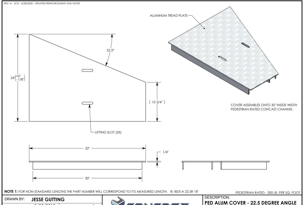
CREATED DATE: 3/22/2010 REVISION LEVEL: A SAVED DATE: 4/28/2020 SAVED BY: jgutting WEIGHT: MATERIAL: 19 LBS. **WELDED ALUMINUM**
