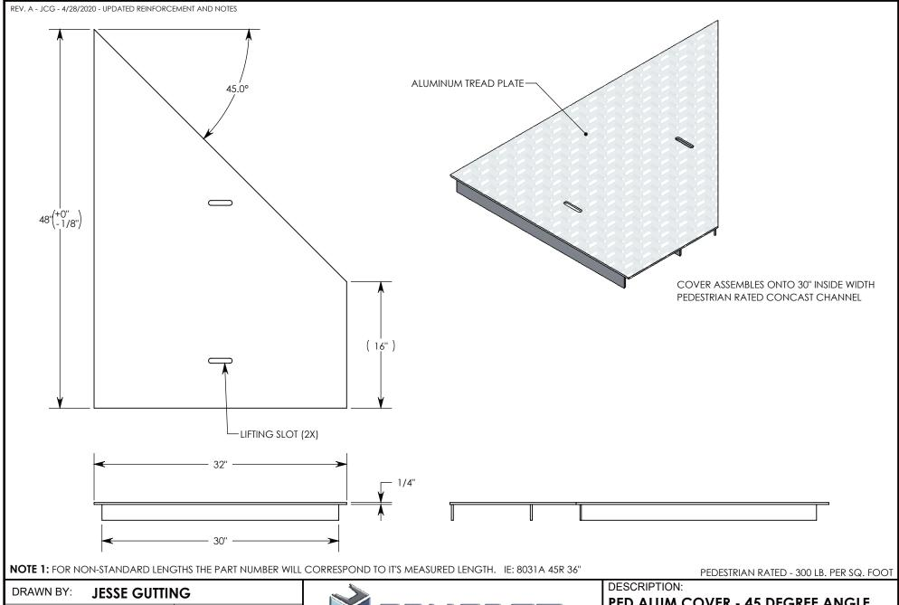
CREATED DATE: 3/22/2010 REVISION LEVEL: 0 SAVED DATE: 4/28/2020 SAVED BY: jgutting WEIGHT: MATERIAL: **WELDED ALUMINUM** 34 LBS.
