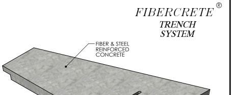
COVER ASSEMBLES ONTO 30" INSIDE WIDTH PEDESTRIAN RATED **PT** CONCAST CHANNEL.
