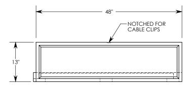
NOTE: FOR NON-STANDARD LENGTHS THE CHANNEL WILL BE SOLID BOTTOM AND DESIGNATED WITH ITS CORRESPONDING LENGTH MEASUREMENT. IE: 8040 32"
