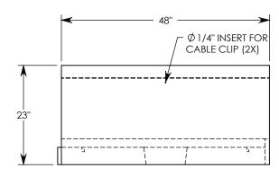
**NOTE 1:** FOR NON-STANDARD LENGTHS THE CHANNEL WILL BE SOLID BOTTOM AND DESIGNATED WITH ITS CORRESPONDING LENGTH MEASUREMENT. IE: 804016HT3 32"
