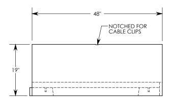
**NOTE:** FOR NON-STANDARD LENGTHS THE CHANNEL WILL BE SOLID BOTTOM AND DESIGNATED WITH ITS CORRESPONDING LENGTH MEASUREMENT. IE: 804016PT 32"
