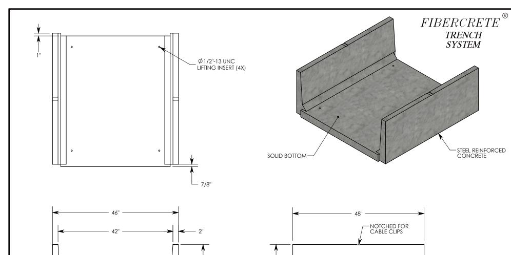
**NOTE:** FOR NON-STANDARD LENGTHS THE CHANNEL WILL BE SOLID BOTTOM AND DESIGNATED WITH ITS CORRESPONDING LENGTH MEASUREMENT. IE: 804016PTSB 32"
