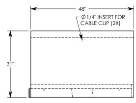
MAX AASHTO H-40 RATED - 64,000 LB. SINGLE AXLE LOAD DEPENDENT ON TRENCH COVER RATING MINIMUM ALLOWABLE SOIL BEARING PRESSURE – H-40: 3,000 PSF; H-20: 3,000 PSF
