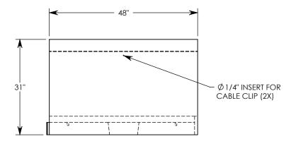
**NOTE 1:** FOR NON-STANDARD LENGTHS THE CHANNEL WILL BE SOLID BOTTOM AND DESIGNATED WITH ITS CORRESPONDING LENGTH MEASUREMENT. IE: 804024HT4 32"
