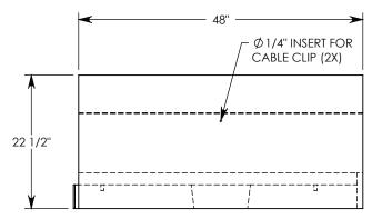
NOTE 1: FOR NON-STANDARD LENGTHS THE CHANNEL WILL BE SOLID BOTTOM AND DESIGNATED WITH ITS CORRESPONDING LENGTH MEASUREMENT. IE: 8040HT 32"
