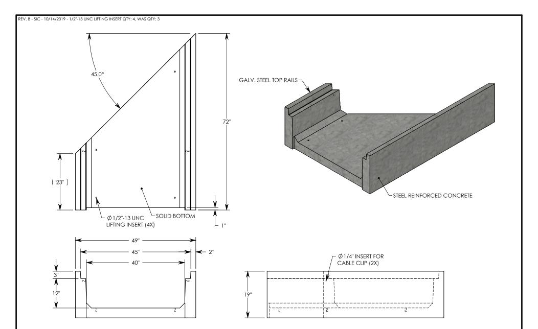
AASHTO H-20 RATED - 32,000 LB. SINGLE AXLE LOAD MINIMUM ALLOWABLE SOIL BEARING PRESSURE – X,XXX PSF
