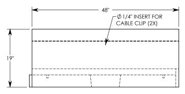
NOTE 1: FOR NON-STANDARD LENGTHS, THE CHANNEL WILL BE SOLID BOTTOM AND DESIGNATED WITH ITS CORRESPONDING LENGTH MEASUREMENT. IE: 8040HT4 32"
