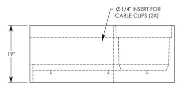
MAX AASHTO H-40 RATED - 64,000 LB. SINGLE AXLE LOAD DEPENDENT ON TRENCH COVER RATING MINIMUM ALLOWABLE SOIL BEARING PRESSURE – H-40: 3,000 PSF; H-20: 3,000 PSF
