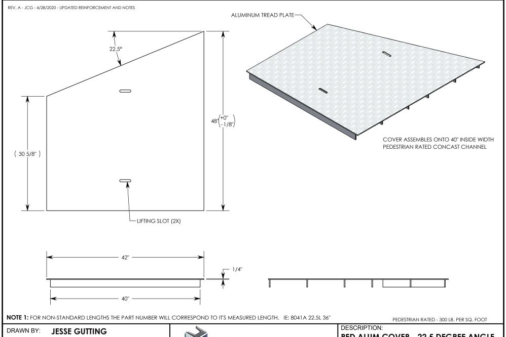
CREATED DATE: 3/22/2010 REVISION LEVEL: A 4/28/2020 SAVED DATE: SAVED BY: jgutting WEIGHT: MATERIAL: **WELDED ALUMINUM** 53 LBS.
