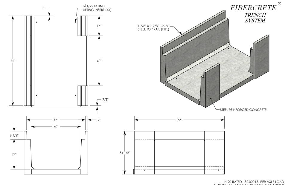
H-40 RATED - 64,000 LB. PER AXLE LOAD WHEN USED IN COMBINATION WITH HTSG40 COVERS
